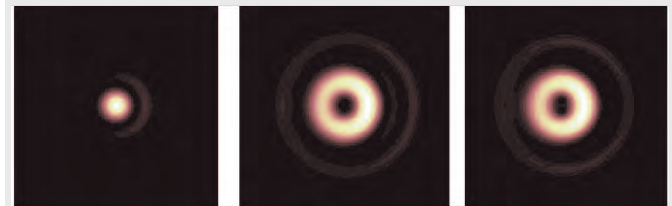
Fig. 2: Effects of a vortex wavefronts on an aberrated field with coma. Left: Single source with no vortex. Center: Single source with m = 2 . Right: two sources with m = 2 . Notice that the dark regions are present and thus we can infer the presence of two close sources.
